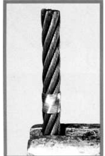
2. Open the rope and broom individual wires. Clean the broom with a solvent or other effective degreaser that does not leave a residue behind. Air or blow dry.
