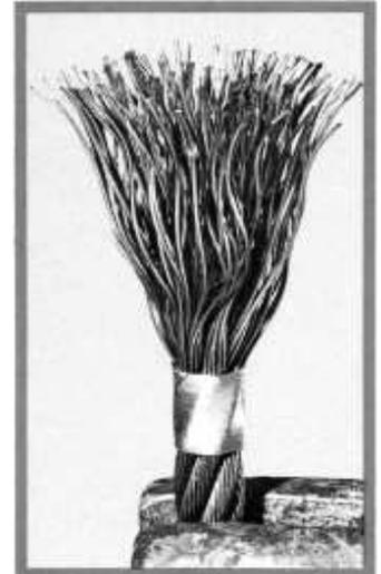
3. Position the broom in the socket, mount the assembly securely, and align the axis of the rope and fitting. Most sockets will be poured vertically, as shown, but larger ones may be filled horizontally (page 4). Seal the socket neck with putty, duct tape or a similar material to prevent leakage. Make sure the socket temperature is at least 18 °C (65 °F) and preferably 25 °C to 30 °C (75 °F to 85 °F). Caution: Socket temperatures above 38 °C (100 °F) may cause premature hardening.
