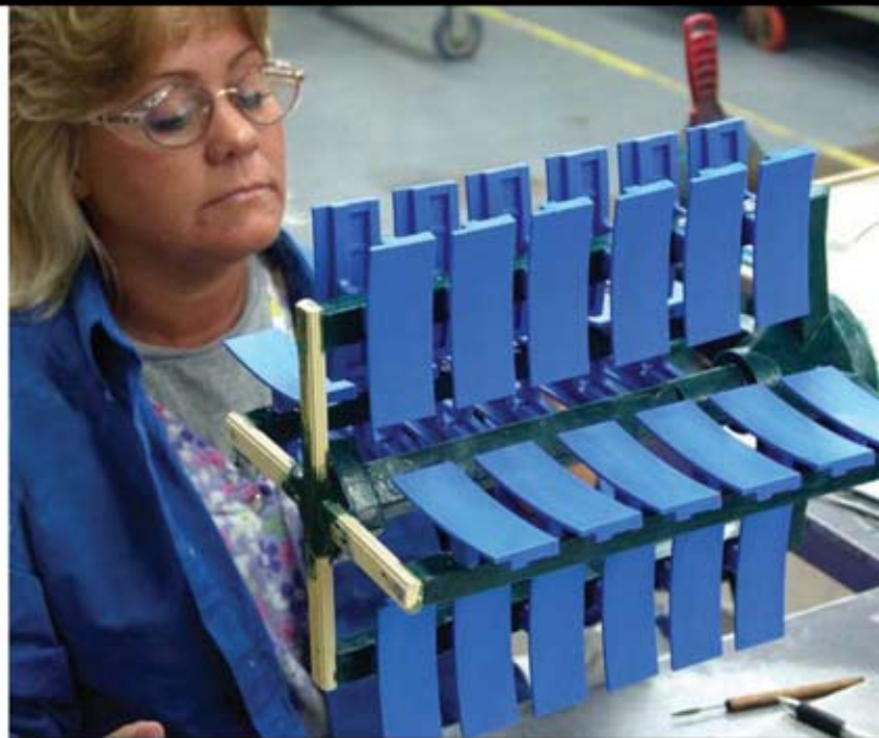
Wax patterns are carefully checked for quality before advancing to the mold dipping process.
